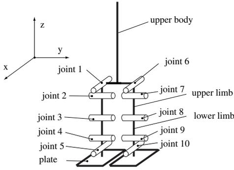
Fig. 1. model of robot of the first step
