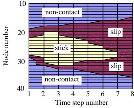
Fig. 7 Calculated contact condition
