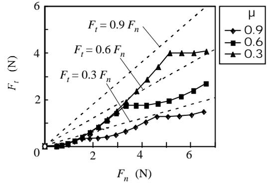
Fig. 10 Normal and tangential force calculated in FE analysis
