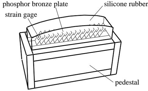
Fig. 4 Top view of finger-shaped sensor
