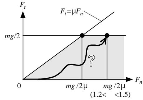
Fig. 2 Change in normal and tangential force for grasping an object
