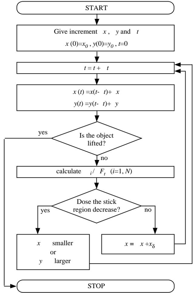
Fig. 9 Flow chart of proposed grasp force control by finger-shaped sensor
