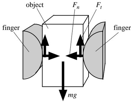
Fig. 1 Force between finger and object for grasping an object
