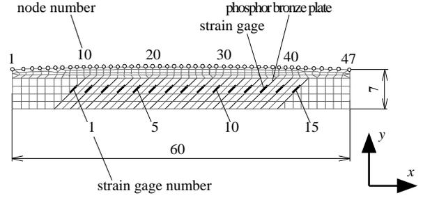
Fig. 5 Finite element model of the elastic finger
