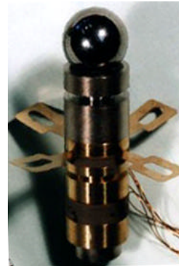
Fig. 7 Picture of a multi-DOF ultrasonic motor
