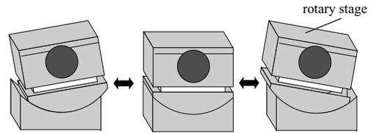
Figure 17: Movement of the rotary stage
