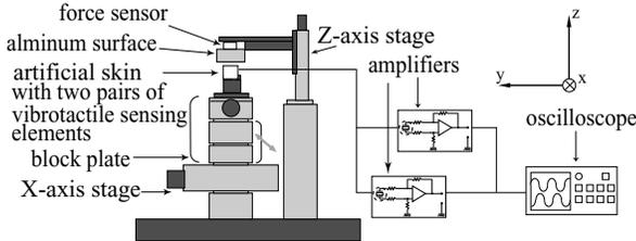
Figure 9: Experimental setup
