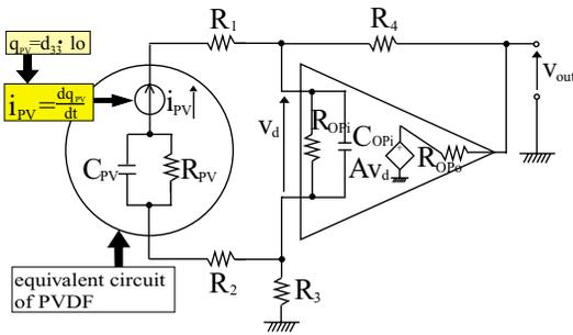
Figure 6: Overall equivalent circuit of the PVDF circuit
