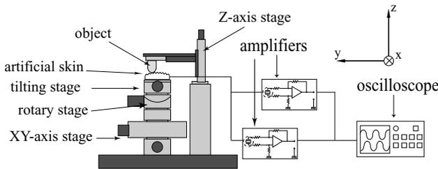
Figure 16: experimental setup
