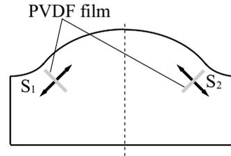
Figure 11: Points and directions for subtracting the stress
