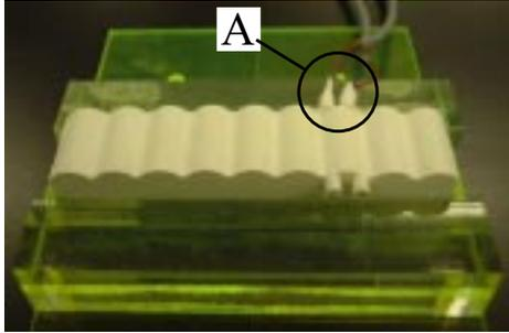
Figure 8: Picture of the manufactured artificial finger skin
