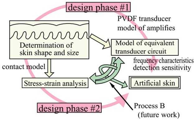
Figure 1: Design process of artificial finger skin
