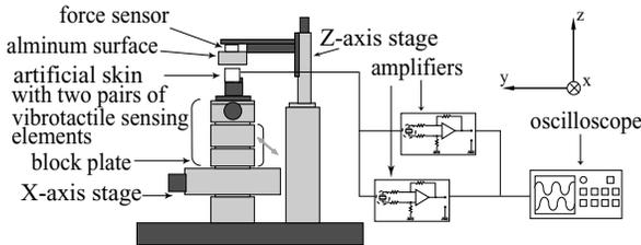
Figure 9: Experimental setup
