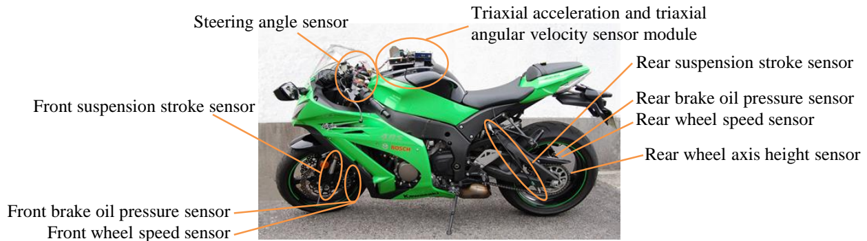
Fig. 1 Test vehicle and measurement equipments
