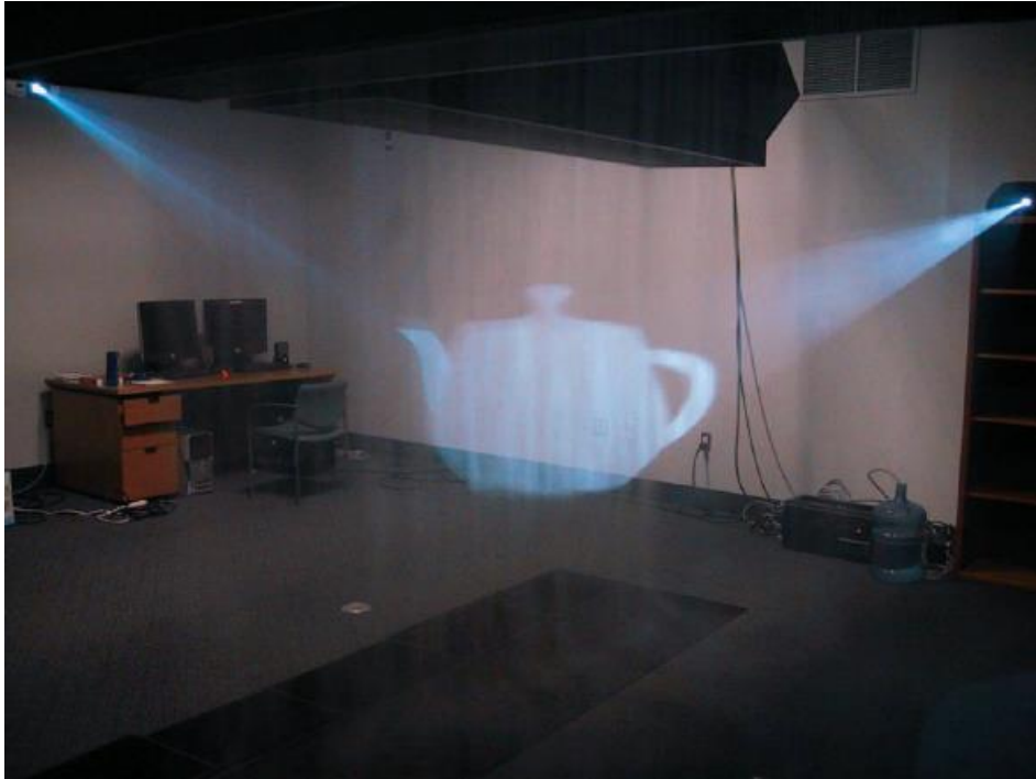
Fig.2-10: Immaterial DFD display using two fog screens
