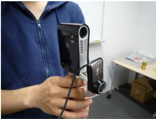
Fig. 2 Prototype of portable AR projection system that consists of portable projector, USB camera and note PC.
