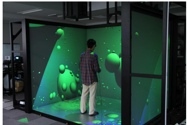
Figure 1: A viewer was operating in an immersive display with 4 screens: KCave.
