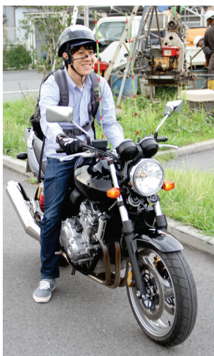
Figure 6: The motorcycle with attached marker bar, and the subject wearing the eye-mark recorder under the helmet.
