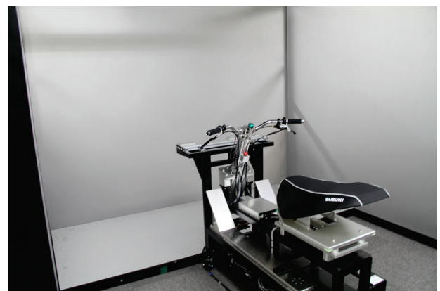
Figure 1: The scooter type motorcycle integrated inside the K-CAVE.
