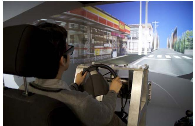
Fig. 6 Created course model was displayed in our immersive car driving simulator.
