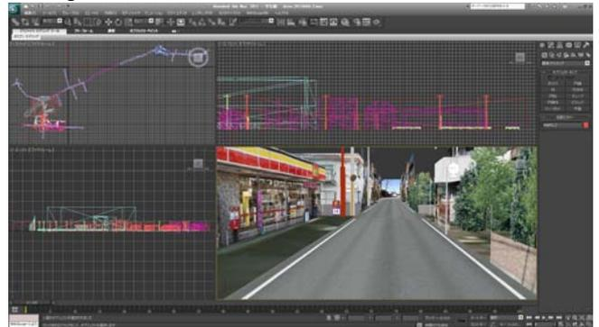
Fig. 5 A course model was created using one of de-facto standard 3D modellers (Autodesk 3ds MAX).
