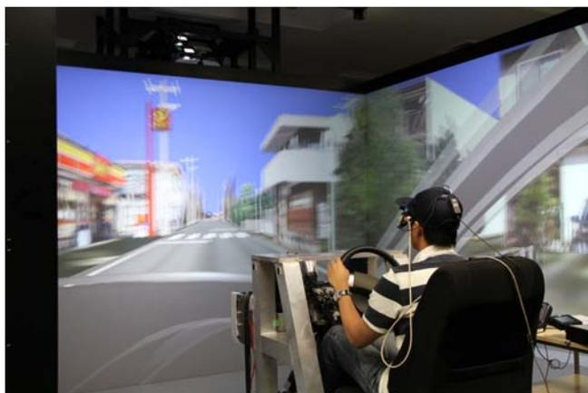
Fig. 1 A driver was driving in the K-Cave Car Driving Simulator.
