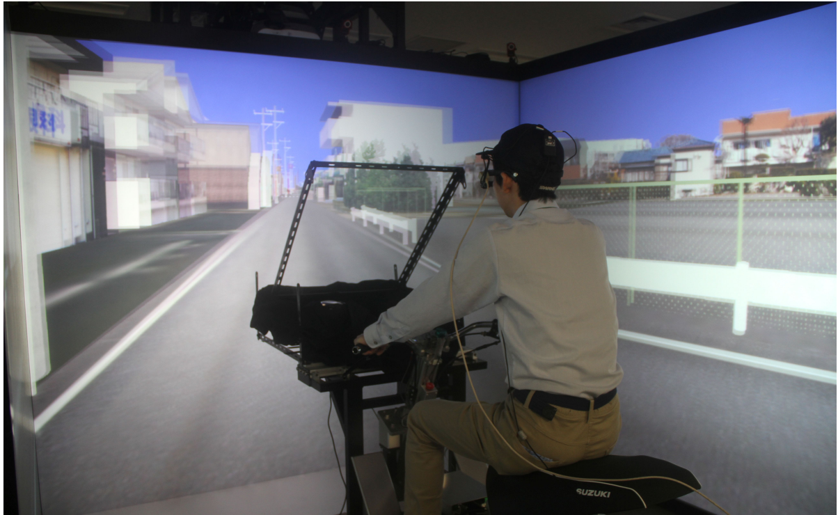
Figure 1 Immersive CAVE experiment environment with head-up display
