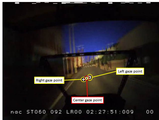
Figure 2 Recorded movie from eye-mark recorder with gaze point explanations
