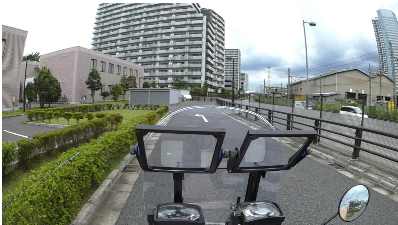
Figure 4 Recorded scenery from a wearable camera showing information presented on the HUD.
