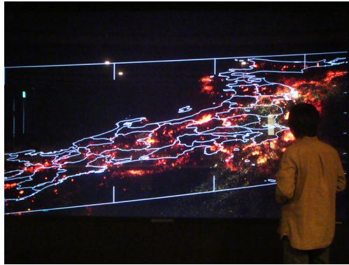
Fig. 6. Visualization of hypocenter data using 4K stereo projection system. User can recognize both each hypocenter data and distribution of whole data.
