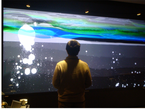
Fig. 7. Integrating visualization data in CDF. The relation between terrain data and hypocenter data are shown.
