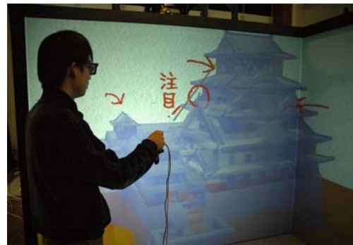
Figure 4. 3D marker used in the virtual space
