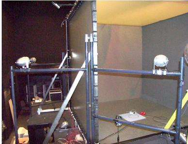
Figure 6 Multi-channel speaker system in the CABIN
