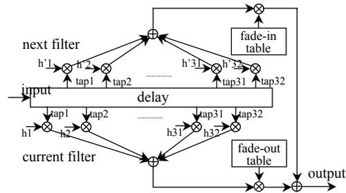
Figure 4 Cross fading method using multi-tap filter
