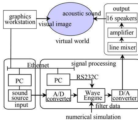
Figure 5 Construction of acoustic display
