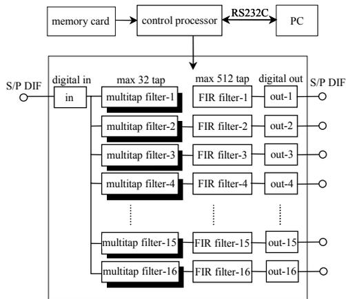
Figure3 Functional diagram of the Wave Engine
