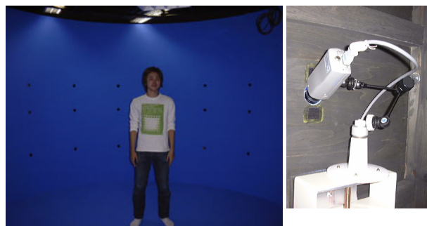
Figure 15. Video avatar studio with multi-camera system
