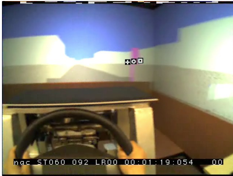
Figure 8. Example recorded image of the eye tracker. The subject's gaze points were marked in the subject's view camera images.
