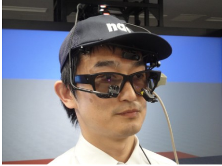
Figure 7. The NAC EMR-9 (an eye tracking system) and polarizing filter stereo glasses for K-Cave were worn simultaneously in our immersive car driving simulator.
