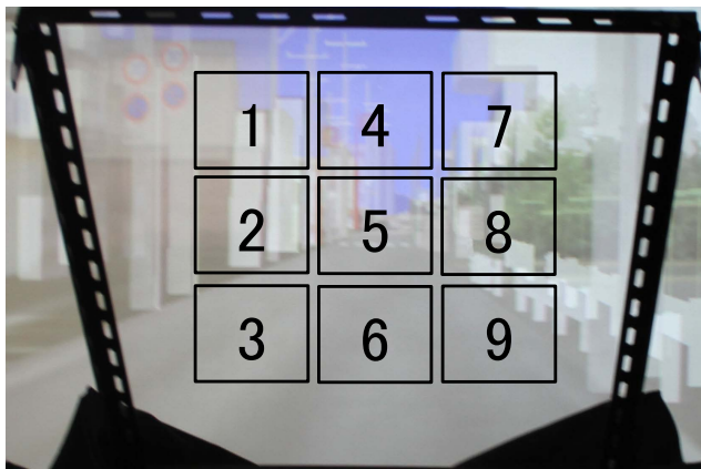
図7 HUD上の提示箇所 Fig. 7 Nine positions on the HUD to evaluate where to present.
