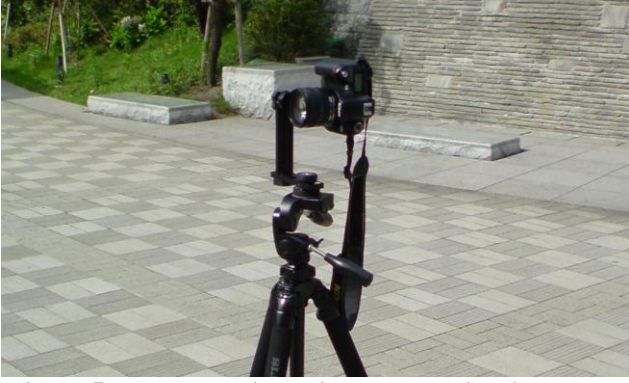
Figure 5. Photographing using panoramic tripod head
