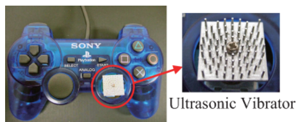
Fig.1 An ultrasonic vibrator attached to game controller.
