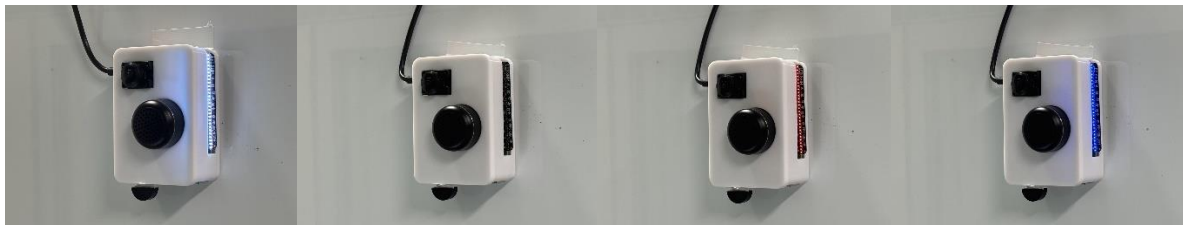
Fig. 3 Light emission pattern of IoT devices (off, white, red, blue).
